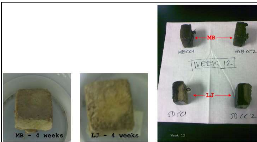
Figure 16 . Biofilm Build Up on Concrete Coupons from Cottonwood Creek and CSD037 at Week 4 and Week 12
